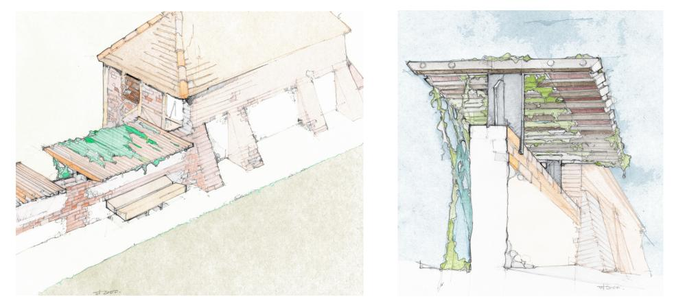
Overhead panels are formed by threading machined timber sections along four stainless steel rods. Using the existing wall's coping as a support these panels offer shade to both the terrace and the sunken garden behind. Climbers are grown in the sunken garden and are trained up cables to the overhead canopy, adding visual interest to the gardens back wall.
