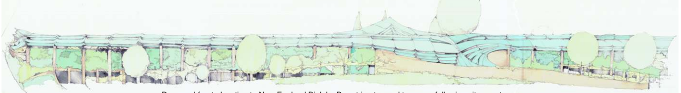
Proposed front elevation to New England Biolabs: Bowstring trussed terraces, following sites contours.
