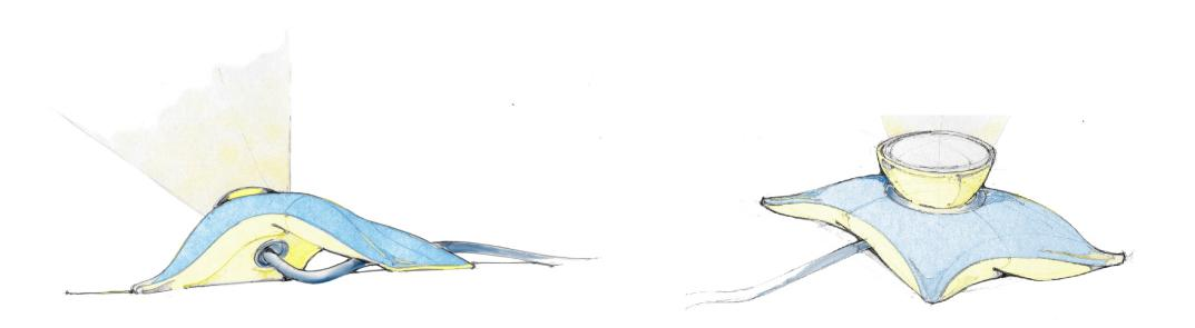
THE BEANIE LIGHT: A tungsten halogen bulb is mounted at the centre of a jell or bean filled sack, allowing the bulb to be angled in any direction.
