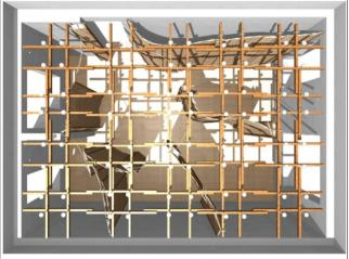
Here our nominal initial arrangement is partially opened up, to allow circulation between different segments of the apartment. This is archived by simply using individual segments as sliding doors.
